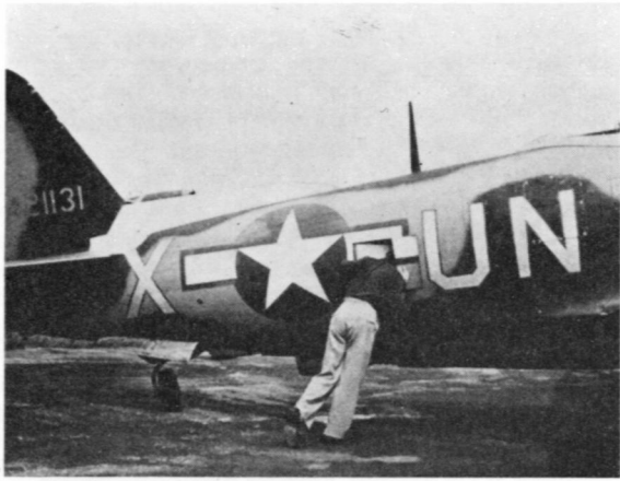
Matt black finished P-47M of 61st FG with unauthorized pale blue outline to 'star and bar'. This was common to all squadron aircraft with black camouflage finish as was the white outlining of code letters. (W. Lanowski)
