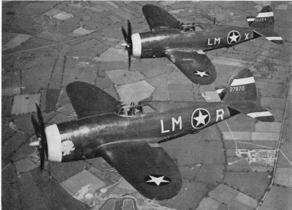
Two early P-47Cs of 62nd FS with code letters. The farther aircraft has unusually small letters, apparently 18 inches high, while 'Happy', LM:R, has standard size 24 inch high letters. (USAAF)
