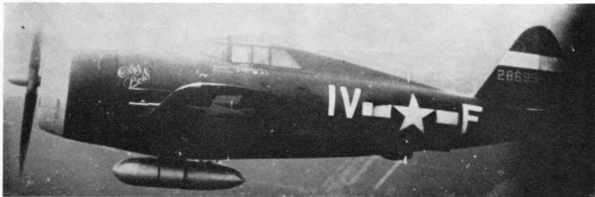
'Oily Boid', a P-47D-5-RE from the 359th FG, collapsing a silver dope impregnated paper type drop-tank. Bands round tank were signal red. (Via R. Hill)
