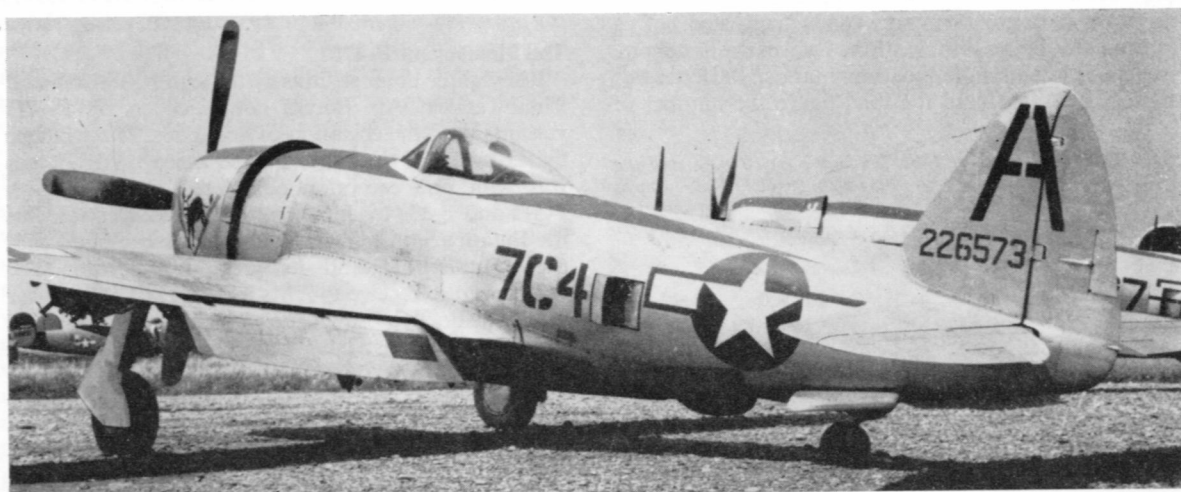
Squadron badge (kicking mule between two lightning flashes) was usually applied to both sides of 347th FS P-47 cowlings. Letter A on tail was a squadron marking. Painted patch on flap is red 'No Step' warning. (S. Staples via R. C. Jones)
