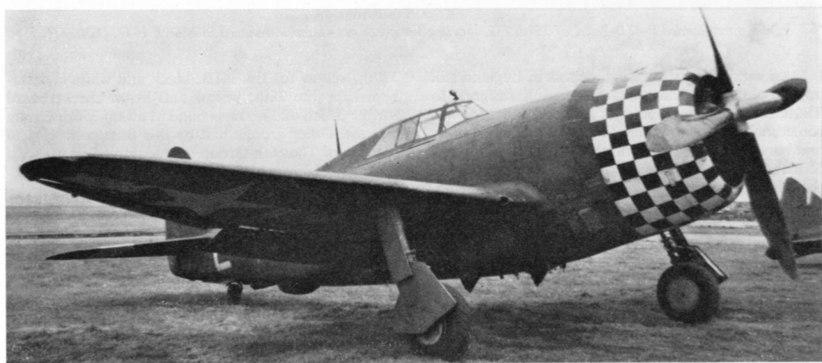
Detail of location of new national marking on a battle damaged P-47D, 42-7905, of 350th FS. Apex of star is centred on skin joint. (USAF)
