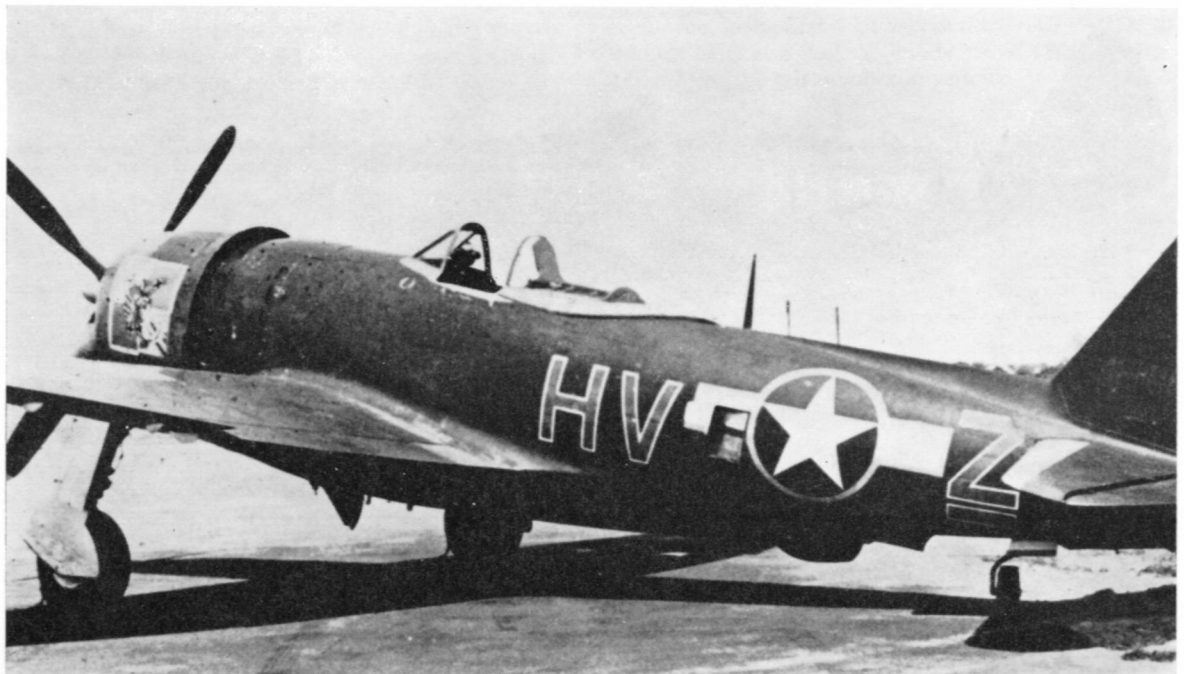
Matt black finished P-47M of 61st FG with unauthorized pale blue outline to 'star and bar'. This was common to all squadron aircraft with black camouflage finish as was the white outlining of code letters. (W. Lanowski)
