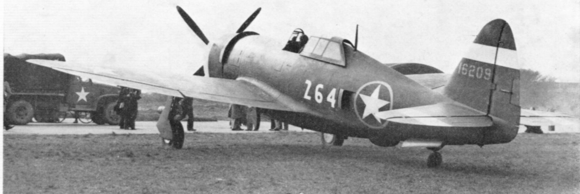
P-47C of the 62nd FS, 56th FG, displaying type recognition bands in white on nose and tail and the yellow outline to fuselage cocarde. Fuselage number is early 'plane-in-group identification marking. (USAF)
