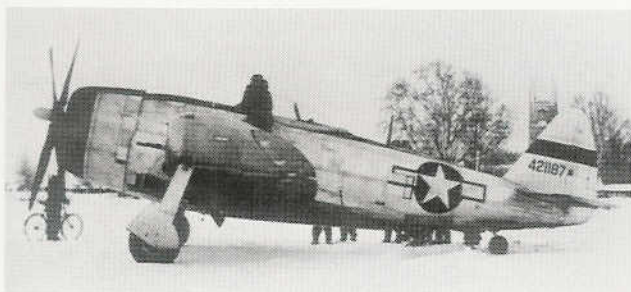
The P-47M, with its R-2800-14W/-57 engine, G. E. CH-5 turbosupercharger, and water injection was used operationally only with the 56th Fighter Group during the closing months of the war. Most were painted in unusual and unofficial camouflage schemes after being received by that unit. This particular P-47M has just arrived in England and has yet to receive a coat of camouflage paint or any unit markings. Also note that the dorsal fin has not yet been added. These were installed after the aircraft arrived in Europe. (USAFM)
