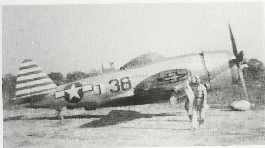
The P-47D-28-RA was produced with the asymmetrical Curtiss Electric propeller. Although added during production of the P-47D-40-RA, dorsal fins were often retrofitted to earlier aircraft to improve lateral stability which was lost when the spine of the fuselage was cut down for the bubble canopy. "Ponnie" was a P-47D-28-RA assigned to the 64th Fighter Squadron of the 57th Fighter Group within the 12th Air Force. (USAFM)
