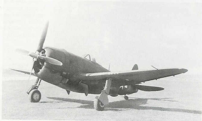
Above: The XP-47J was a project to evaluate the fan-cooled R-2800-61 engine. Initial plans called for an Aeroproducts counter-rotating propeller, but a standard four-blade propeller was fitted. The XP-47J program was ended in favor of the XP-72 covered below. The art on the cowling is an early rendition of Superman. (USAFM)
