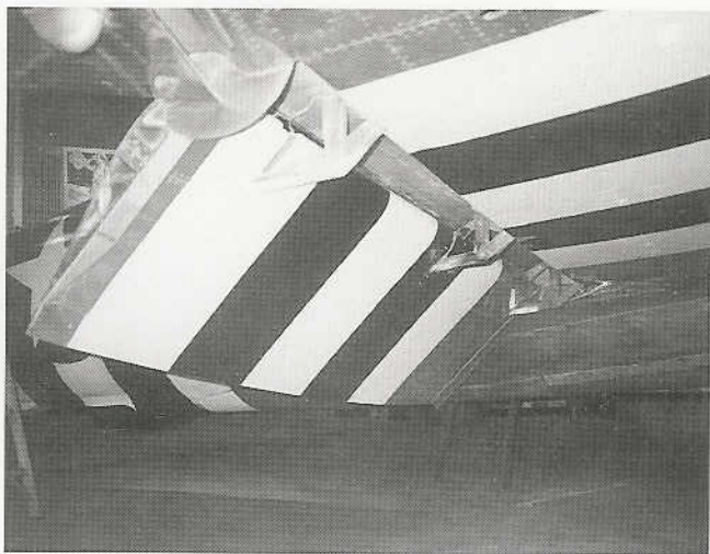
This is the same flap shown at left as viewed from below. The three large hinges are clearly visible.
