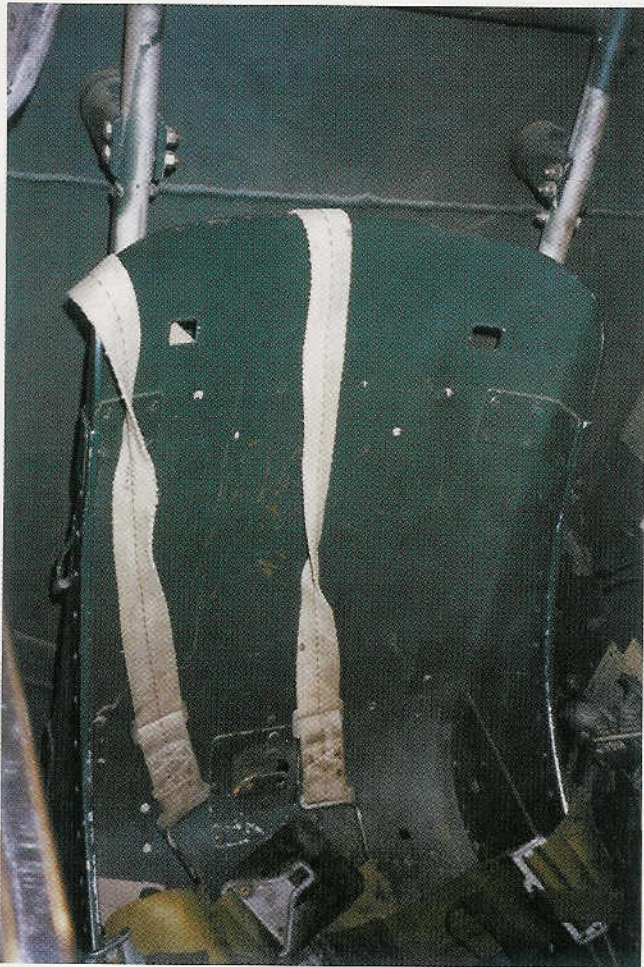
The seat was also painted the Dull Dark Green color. Note that the shoulder straps are off-white, while the lap belts are khaki.
