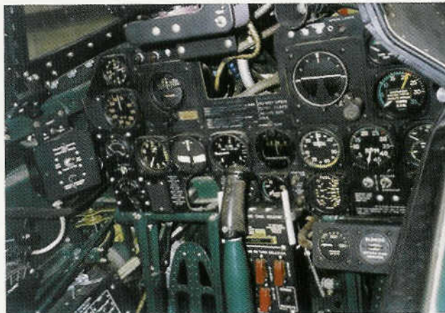
The instrument panel in the P-47M was very similar to that in late P-47Ds.
