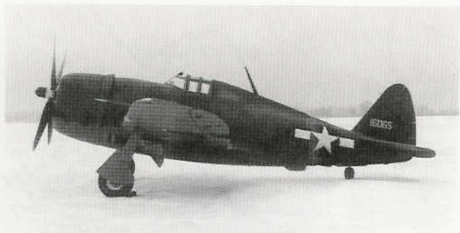
The last production P-47B was fitted with the clamshell cockpit entry door like that found on the XP-47B and the first two production P-47Bs. Notice that the original rear window design was also used. This aircraft served as the test bed for a fighter with a pressurized cockpit, and it was redesignated the XP-47E. The Hamilton-Standard propeller was also evaluated on this Thunderbolt, and it was fitted by the time this photograph was taken in the snow at Wright Field. (USAFM)
