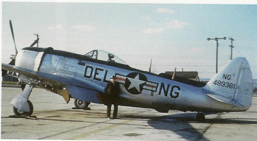
Right: An immaculate F-47N from the Delaware Guard has nothing to indicate its unit except the lettering on the sides of the fuselage. Post-war Thunderbolts were often painted with silver dope which helped to seal the skin and prevent corrosion. (Boseth via Menard)
