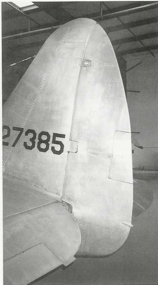
Rudders on P-47Bs were originally covered with fabric, but this was changed to a metal-skinned rudder on all subsequent Thunderbolts.
