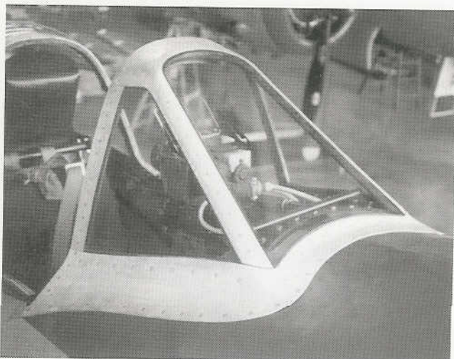
The windscreen used with the bubble canopy was completely different than that used with the earlier framed design. The front flat glass was bulletproof to provide protection for the pilot.
