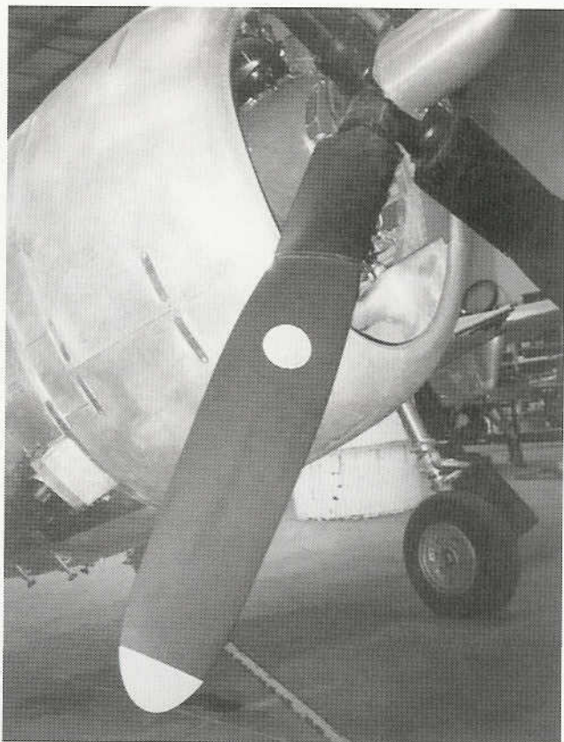
Above: Curtiss Electric also introduced two different propellers with wider chords, and these were first used in production on the P-47D-23-RA. One design looked very much like the Hamilton-Standard Hydromatic propeller, except that it was fitted with cuffs. This propeller was known generally as the Curtiss Electric symmetrical paddleblade propeller, and it was 13' 1" in diameter. (USAFM)
