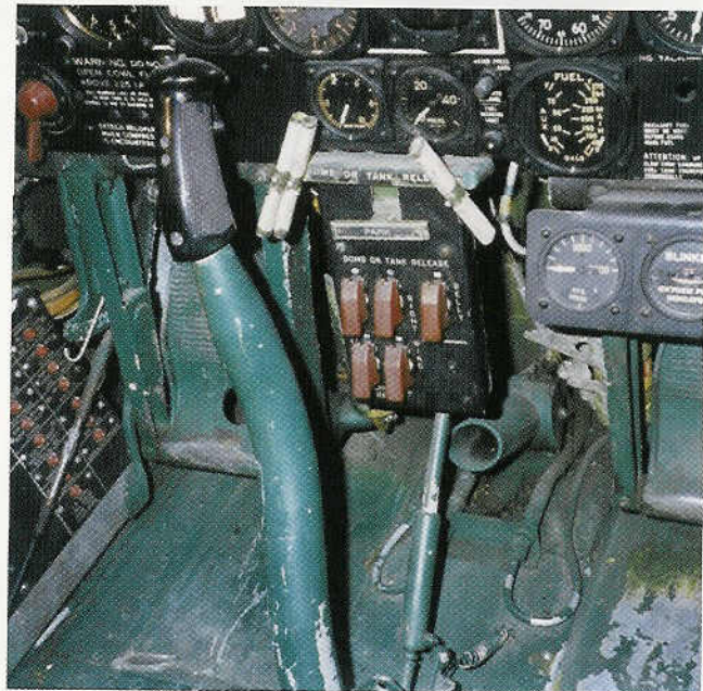
The control column and the rudder pedals were also Dull Dark Green. Note that the floor is smooth rather than being corrugated.
