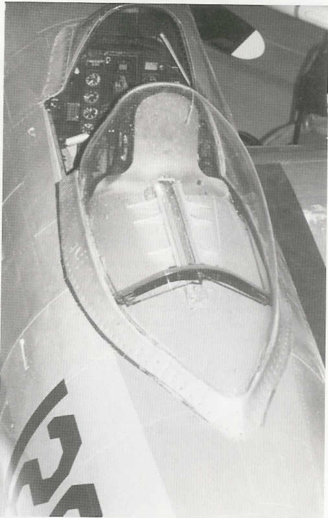
With no spine on the aircraft, a different type of rear protection had to be provided for the pilot. Armor plate was placed just behind the seat to protect the pilot's head and shoulders. This view also provides another look at the center slot and brace.
