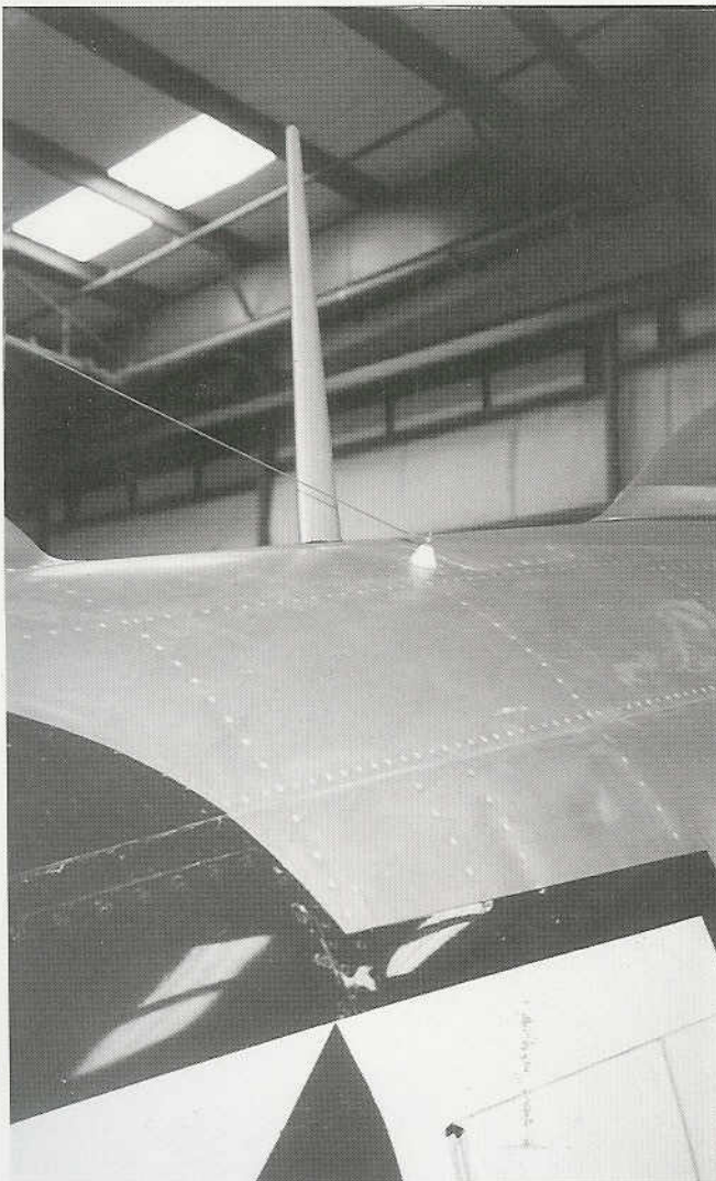
The antenna wire began at a point near the top of the vertical tail and entered the fuselage just to the right of the antenna mast.
