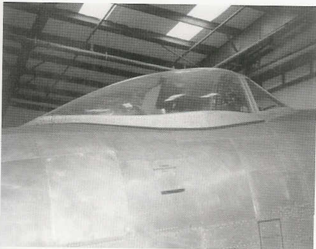
Realizing the importance of seeing the enemy first in both offensive and defensive aerial combat, bubble canopies replaced framed designs on many allied fighter types. The P-47 was no exception, and the bubble canopy shown here became standard on the P-47D-25-RE and the P-47D-26-RA. This changed the overall appearance of the aircraft considerably, but more importantly it increased the pilot's visibility by a significant margin.
