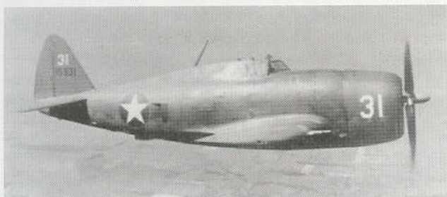
The P-47B could be identified by the radio mast on the spine which was angled forward. While a few were assigned to the 56th Fighter Group, P-47Bs were not considered suitable for combat. In 1944, they were redesignated RP-47Bs with the "R" standing for "Restricted."
