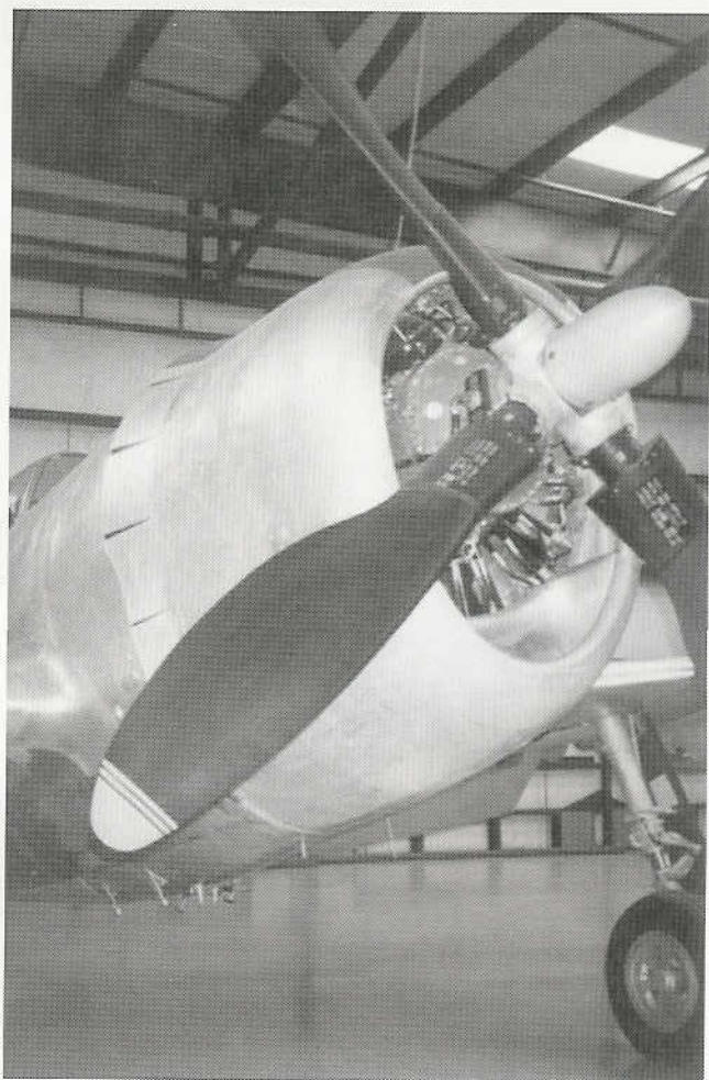
Above: The other Curtiss Electric paddleblade was asymmetrical, because the broadening of the blade's chord was much more pronounced along the trailing edge. Like the symmetrical propeller, it was also 13' 1" in diameter. Most published drawings of this propeller show this feature incorrectly, because they do not illustrate that the broadening of the trailing edge tapers as it approaches the tip rather than remaining almost constant. (USAFM)
