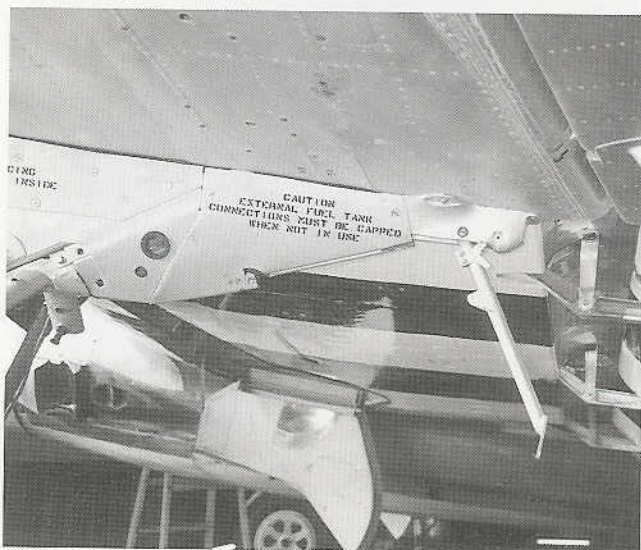
The bar could be rotated down around a hinge on its aft end to provide bracing for an external fuel tank.
