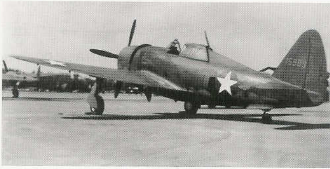
P-47Bs had cowl flaps that extended down to approximately the centerline of the fuselage. None of them had the eight-inch fuselage extension or the bulged keel which were introduced on later versions. This particular aircraft was one of a few P-47Bs modified to carry cameras and serve in the reconnaissance role. These aircraft were initially called RP-47Bs, but this designation was later used for all P-47Bs to denote a restricted flying status. (USAFM)
