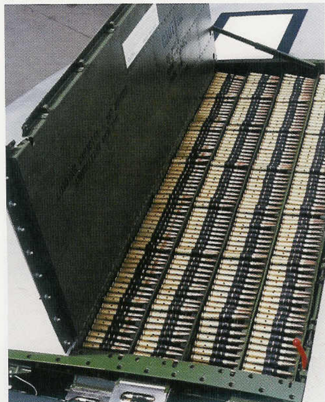
The .50-caliber ammunition was loaded in four parallel trays outboard of the guns. (Ethell)
