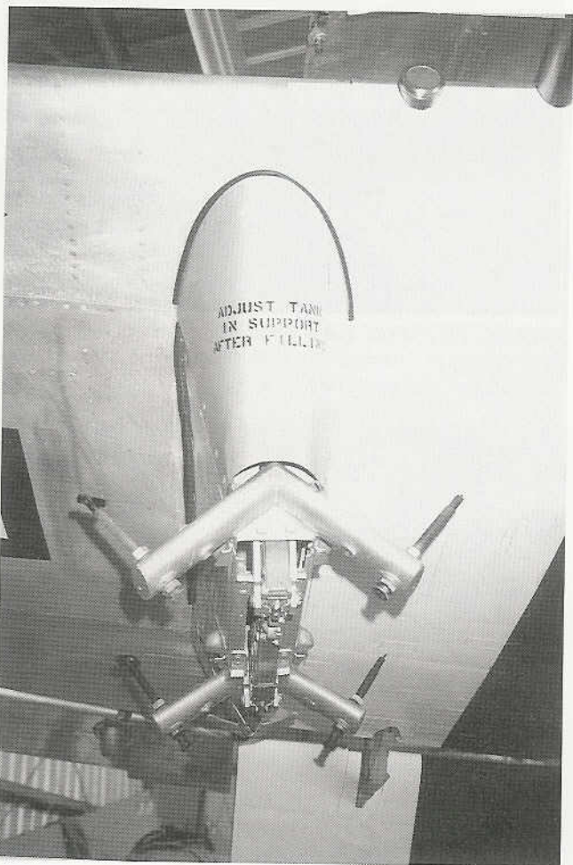
A front view provides a good look at the anti-sway braces.
