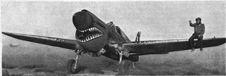
A Kittyhawk Mk. Ia (P-40E-1) of No. 112 "Shark" Squadron, R.A.F., at Sidi Heneish airstrip in 1941. The piratically-bearded warrior sitting on the wing provided "eyes" for the pilot during taxiing; the cowling of the Allison engine effectively blocked forward visibility from the cockpit.
