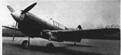
The Curtiss H87A-1, or Kittyhawk I; the first twenty aircraft mounted a wing armament of four .50 calibre machine guns.
