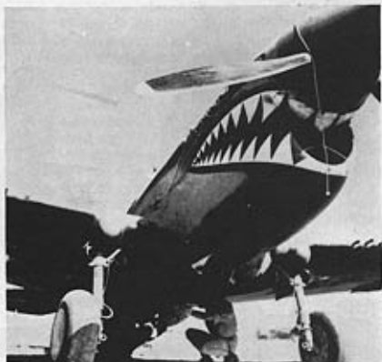
Unusual armament visible on Mk. Ia AK772, GA-Y of No. 112 Sqn. at Gambut Main in June 1942; two 250 lb. bombs mounted in tandem under the centre-section. Note also plugged exhaust ports, with cord linking individual plugs. (Photo: via R. Ward)
