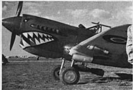
Kittyhawk Mk. III FR864 GA-M, flown from Pachino/Agnone in August 1943 by Squadron Leader Illingworth. Note bomb load; two 250 lb. under fuselage and four 40 lb. anti-personnel under wings. (Photo: via R. Ward)
