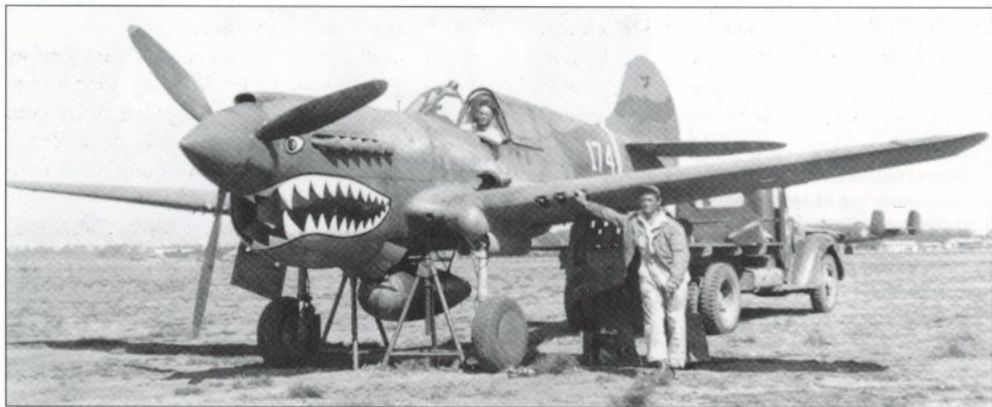
Armourers of the 75th FS boresight the guns of P-40K 'White 174' at Kunming in early 1943. Dark green overpainting of the national insignia and the serial number is clearly visible on the fuselage and tail, as is the 11th BS B-25 parked in the background
