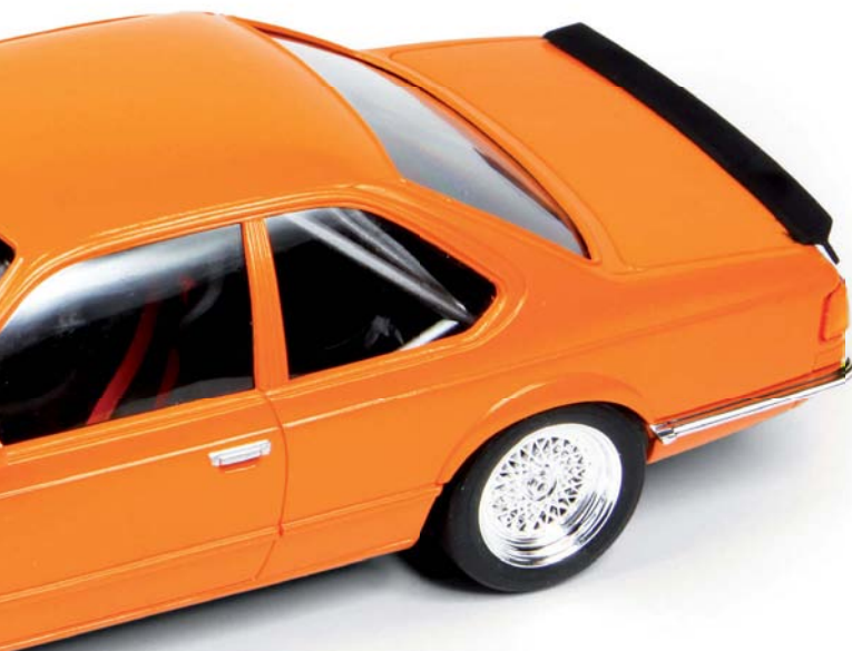
▲ A quick and easy way to simulate glossy electric tape is to use strips of masking tape, 'painted' with a felt pen.
