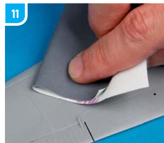
▲ If pressured too hard, the rivets will stand out and would benefit from light sanding with fine abrasive paper.
