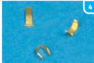
▲ Three-part tool holders are very common on German World War Two vehicles.
