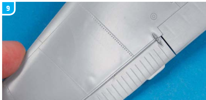
▲ The result is a neat row of circular rivets. The procedure is slow and can be tedious, but rewarding in the end.
