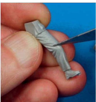
▲ Mould seams on plastic or resin figures are easily scraped away with a hobby knife, followed by careful sanding.
