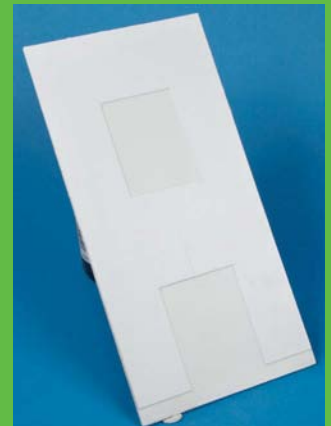
▲▼ An easy way to create different surface levels on plaster buildings is to make a pattern in the plastic mould. The result is a neat raised board around the base, door opening and window.
