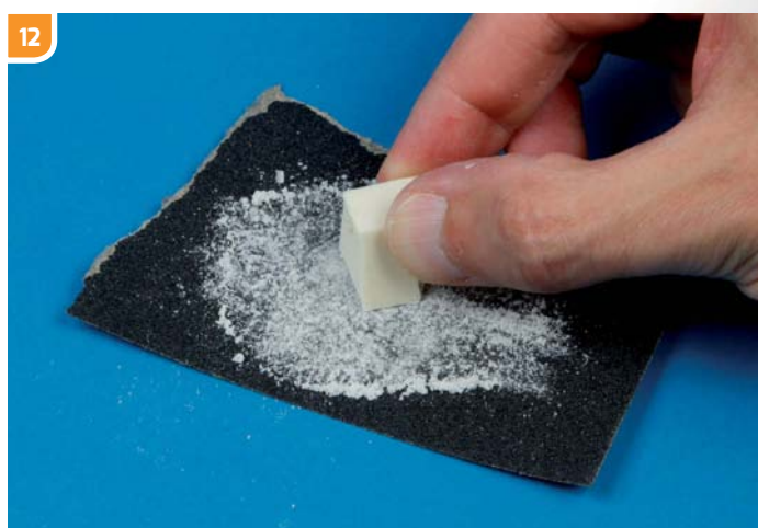
▲ Flat areas such as on this stowage box are best sanded in a circular motion while on a flat surface.
