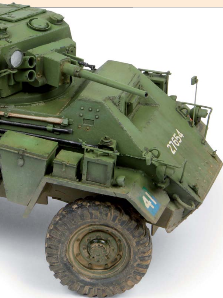
▲ One of the mudguards was damaged slightly so styrene strip was cut to the proper length and glued along the edge. Putty was also needed to finish the task.
