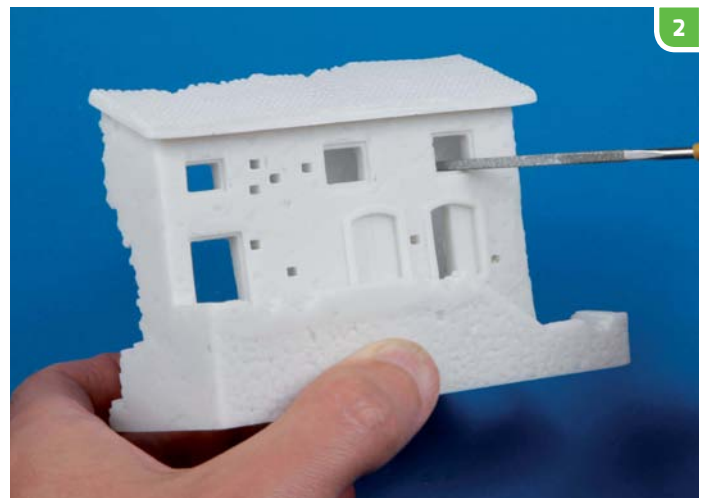
▲ Minor clean-up was needed to remove slight casting seams and excess resin. This was done quickly with a diamond file.
