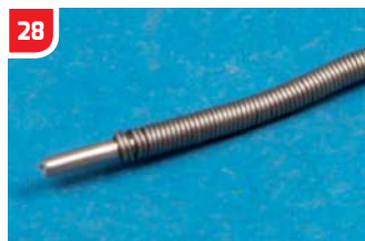
▲ CA glue helped to secure the thin wire to prevent it from sliding off the thicker core.
