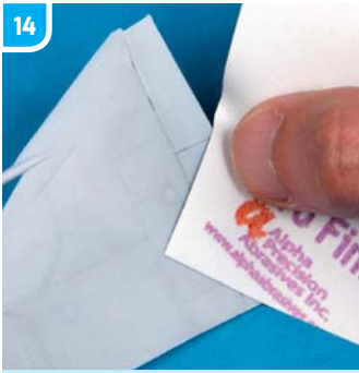
▲ The raised lines were sanded until they were barely visible but still could serve as a guide for new panel engraving.
