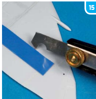
▲ Again, the useful Dymo tape acted as a guide for the rivet scriber. It also protected the surface should the scriber slip.
