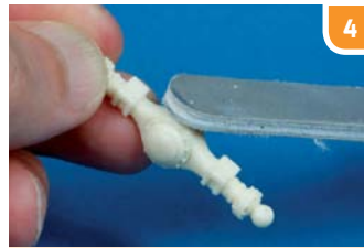
▲ A sanding stick or abrasive paper can then be employed to smooth the seam.
