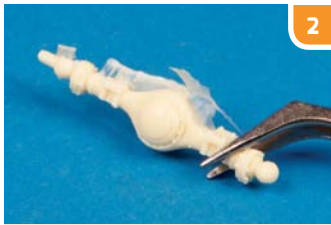
▲ It's not uncommon to see excess resin, similar to flash that can appear on injection-moulded parts.
