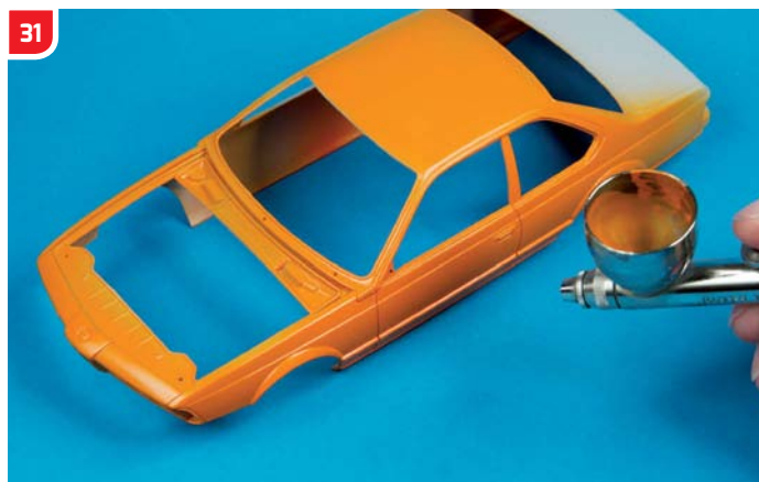
▲ The car body was airbrushed with Tamiya acrylics in several thin layers to obtain a smooth finish.
