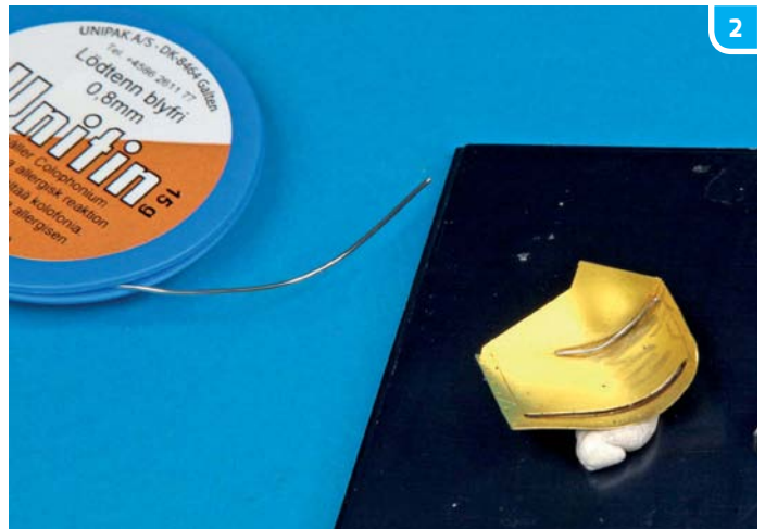
▲ The fender was placed onto a metal plate with the help of Blu-Tack, and a string of solder was placed onto the seam. Flux was first brushed onto the seam itself.
