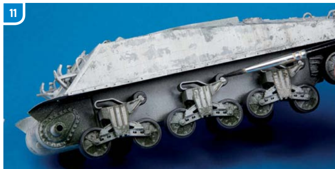
▲ The rubber areas of the running gear were painted with black-grey acrylic paint.
