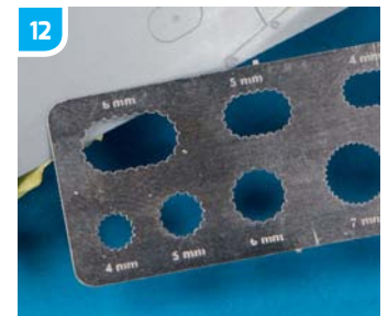
▲ Templates for circular shapes were also included in the set, and were of great help when making rivets around service hatches.
