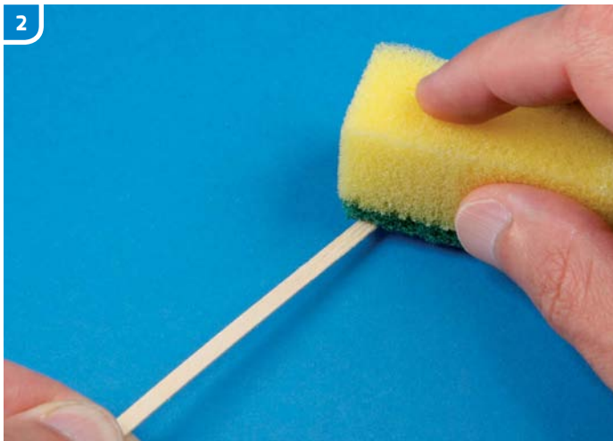
▲ Scotch-Brite was then used to create a finer grain and to even out the torn edges of the planks.
