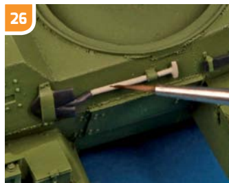
▲ On-vehicle tools were also hand painted. As seen here, the first layer of sand yellow is being applied on the wood areas, and black for the metal.
