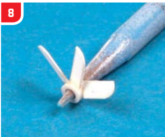
▲ The blades were glued at an angle towards the shaft centre. Once all were in place the fan was given a coat of primer.
