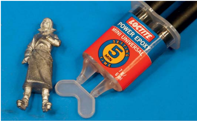
▲ For metal parts, it's necessary to use cyanoacrylate or epoxy glue. Metal pins can also be inserted between the kit parts for a stronger bond.
