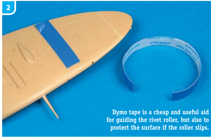
▲ The roller is slowly pushed along the Dymo tape with gentle and constant pressure. Tests should be conducted on a spare model before starting.
