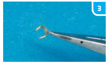
▲ Fine tweezers are absolutely vital for handling and bending small PE items, such as this clasp.
