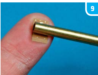
▲ The hatch was held against a finger and formed by rolling, with the help of a brass rod.
