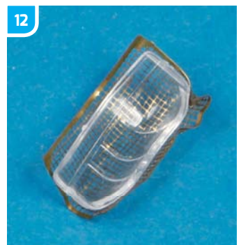
▲ The mesh was pressed around the kit part, which served as a useful template.
