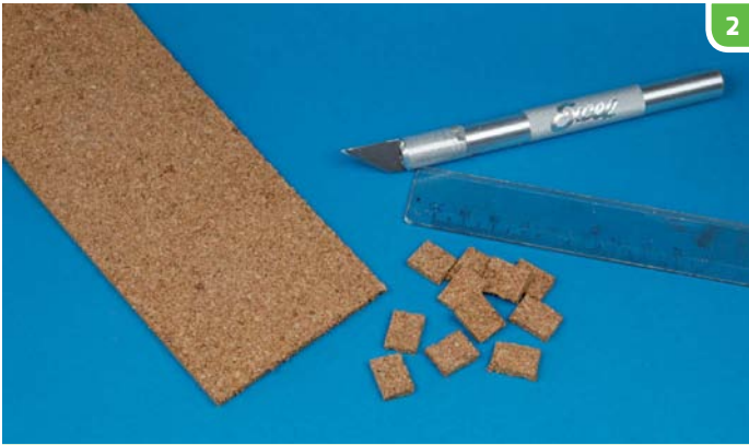
▲ Cork is very easy to work with. Individual stone slabs were cut from a 2mm-thick sheet with a regular hobby knife.
