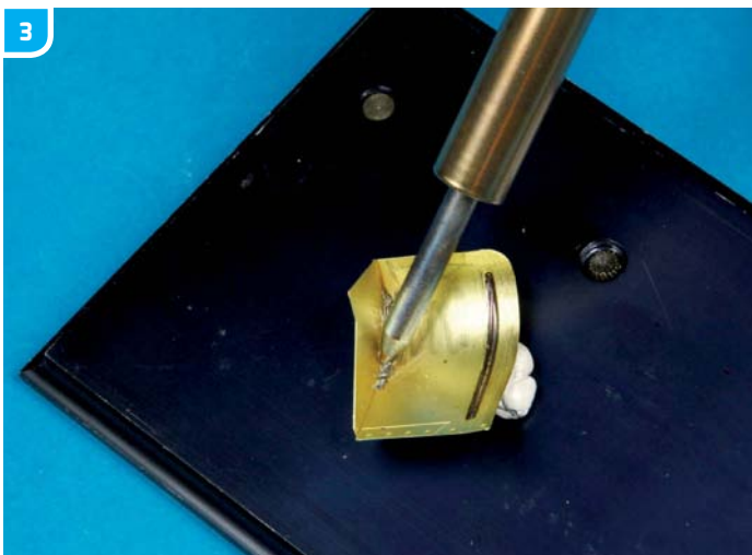
▲ The soldering iron was then placed just over the solder to melt it, and then gently pushed into it to smooth it out.
