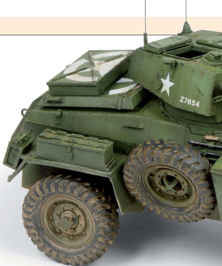
▲ Minor air bubbles and imperfections on the surface were filled with putty and sanded. This is a common task with resin kits.
