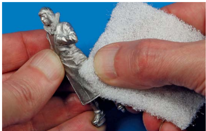
▲ Metal figures are cleaned up with Scotch Brite, used in a polishing motion.
