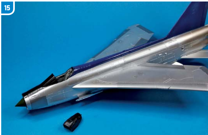
▲ The anti-glare panel was then carefully masked and painted satin black, together with the canopy.
