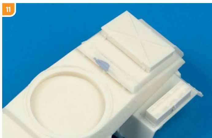
▲ Minor air bubbles and imperfections on the surface were filled with putty and sanded. This is a common task with resin kits.
