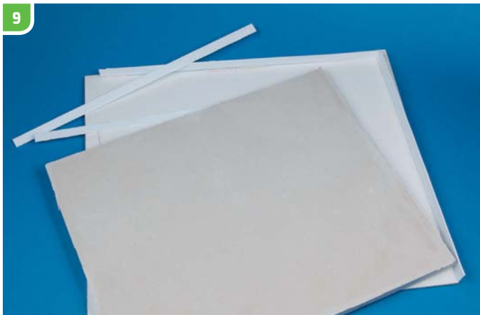
▲ Plaster was simply poured into the mould and, when dry, the sides were snapped off. The plaster sheet could then be removed.
