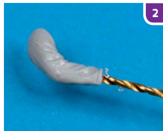
▲ The arm is then drilled out with a small bit in a pin vice. Take care not to crack the edge.
