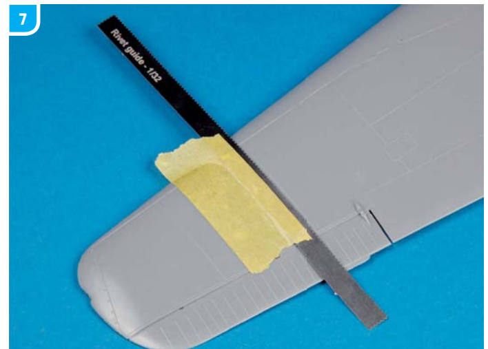
▲ The steel guide in this set from Model Design Construction has a saw-tooth pattern at the edge, to ensure the rivets are set at the correct distance.
