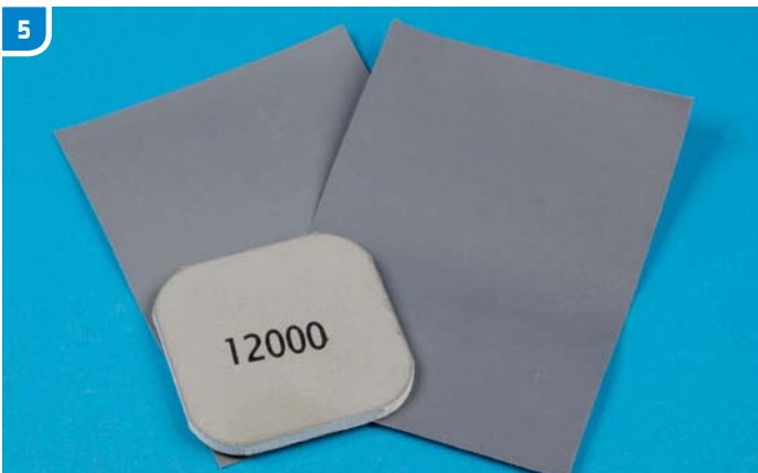
▲ Abrasives and sanding pads with very fine grades were used to polish the first primer coat and correct the flaws. A second layer was then sprayed and also lightly polished.
