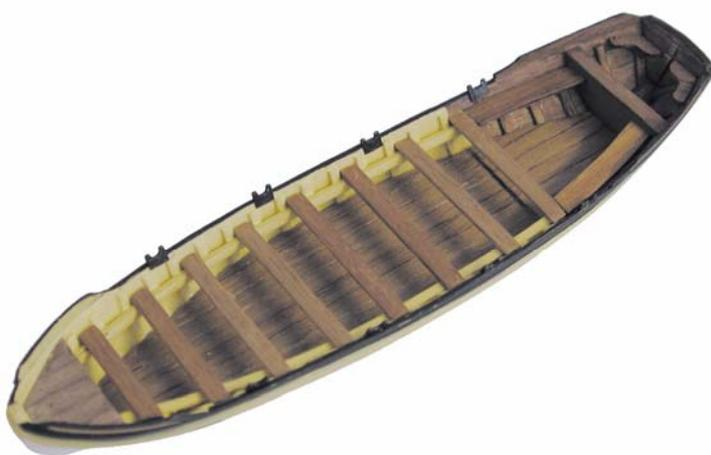
Internal hull detail, note fore raised deck
