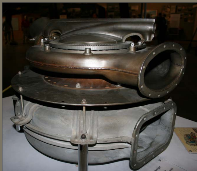
Complete supercharger including compressor chamber as displayed at The National Museum of the Mighty Eight Air Force, Savannah, GA.
