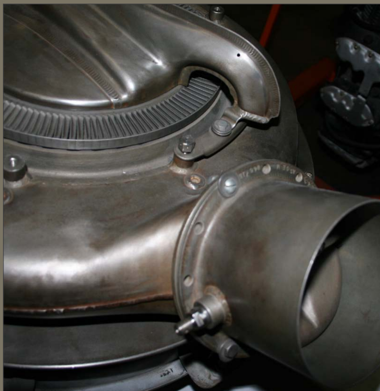
Engine No.4 Supercharger on the B-17G „City of Savannah“, restored in The National Museum of the Mighty Eight Air Force.
