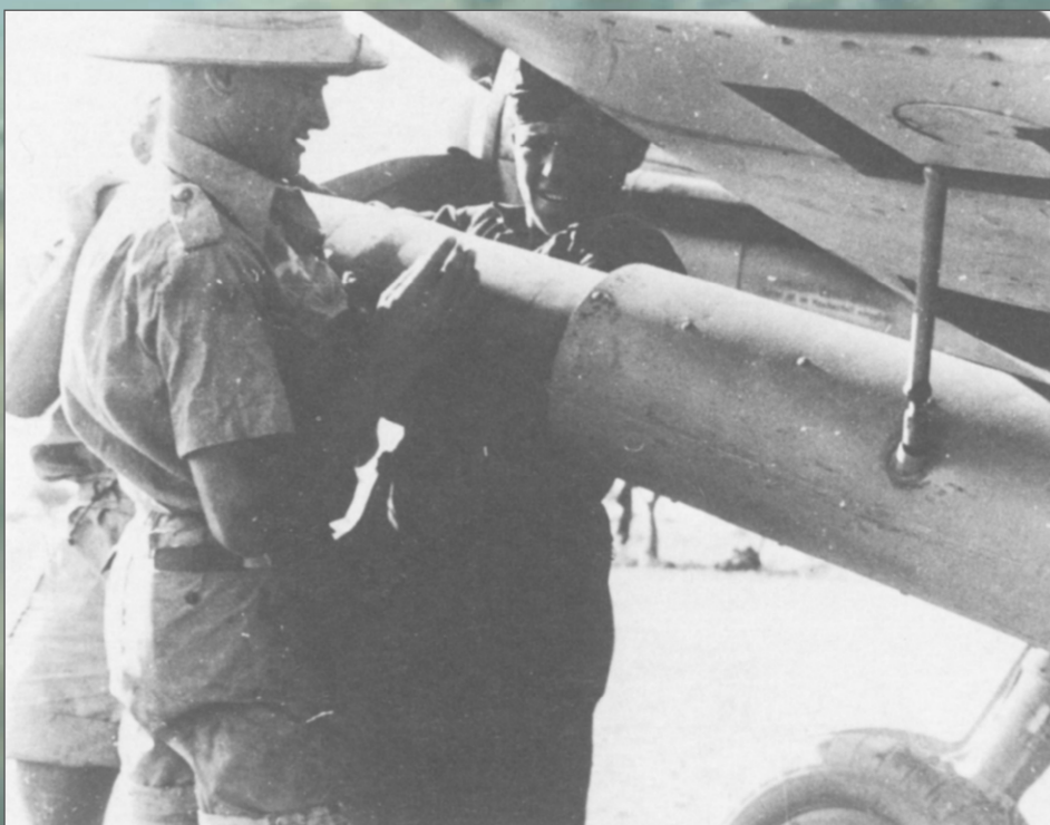
WGr.21 installed on Bf 109G-6.
