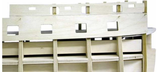
Once that you are happy with the positioning, pin and glue into place, remove any excess from the front of the pattern so that it is flush with the front of bulkhead 1. Repeat the procedure with the opposite pattern.
