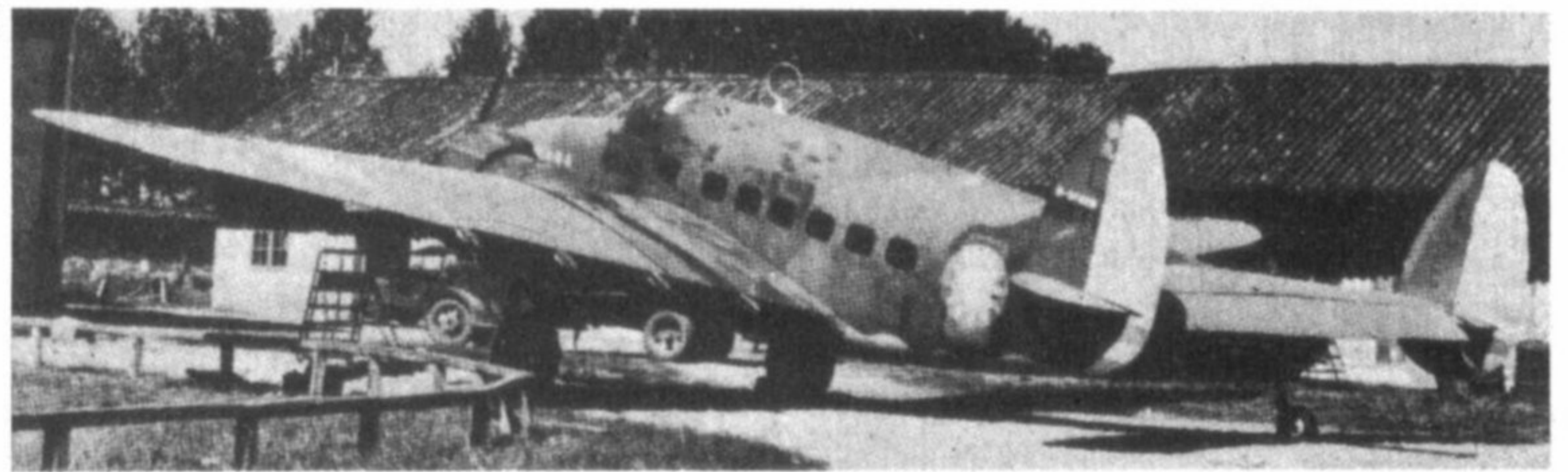
2 Hudson IIIA becomes A-29 (USAAF) and PBO-1 (USN). An early American Services' A-29 with Boulton Paul turret fitted; in service use, the USAAF's anti-submarine Hudsons did not carry the power turret though the Navy's Hudsons did. No. 6 window to the rear has beam gun position addition of two field-of-fire restriction fences. (Photo: Lockheed, ref. Y6360)
