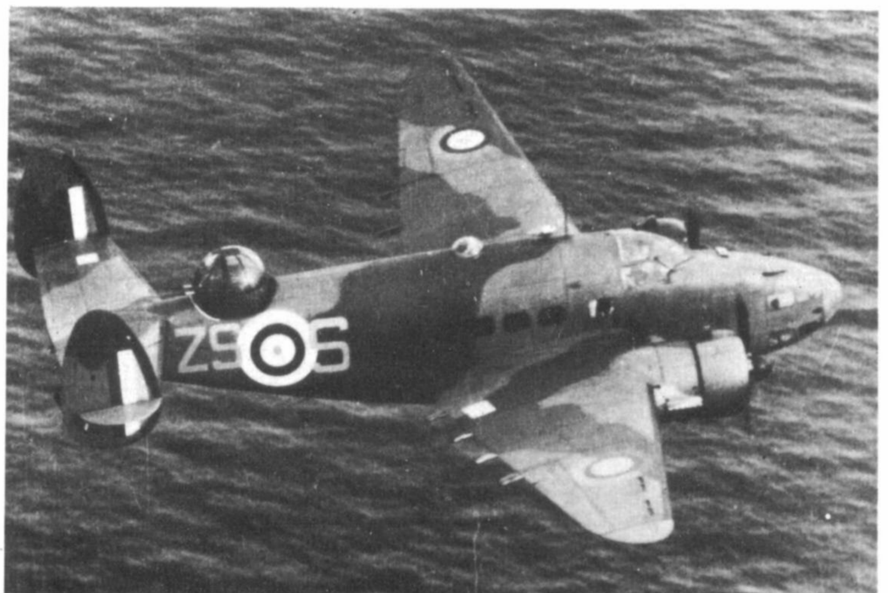
Mast-head-height. An unidentified Hudson Mk I of 48 Squadron (ZS) shows off the camouflage pattern from above. Yellowish paint squares on wing and tail-plane are presumed to be gas-detector panels. In the early part of the war, all military vehicles had to carry such squares or diamonds. ASV Mk I on nose and wing/engine areas but no dorsal mast visible. (Photo: IWM, ref. CH1919)
