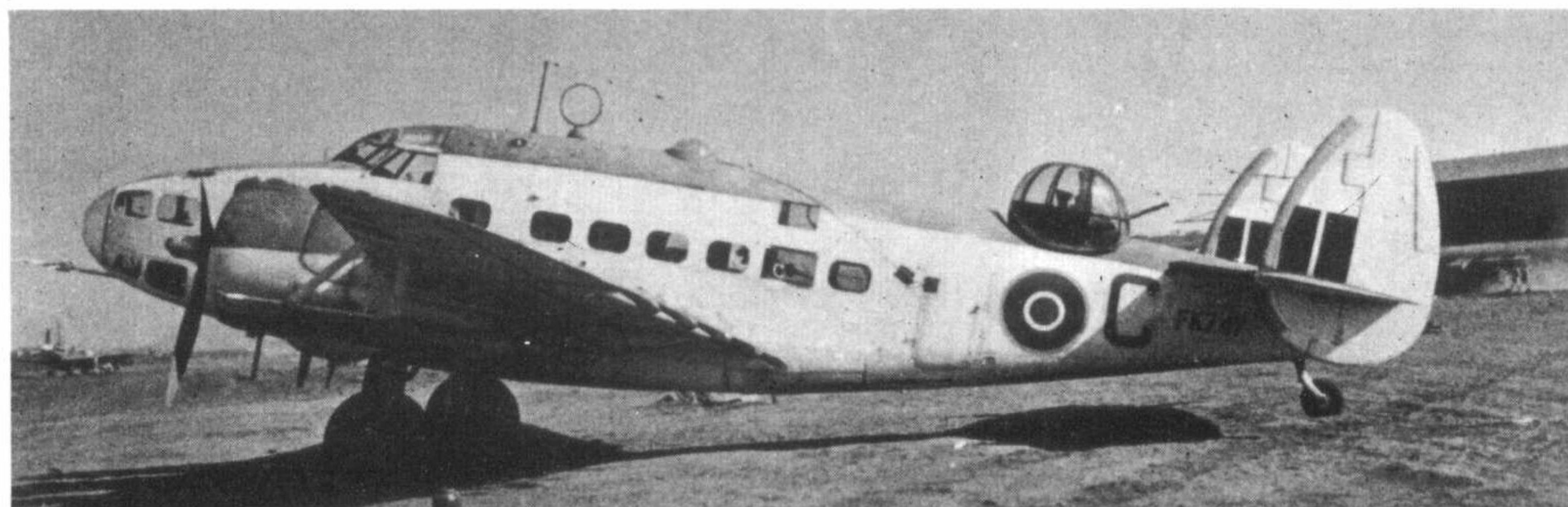
Hudson Mk IIIA (FK747) of No. 48 Squadron, RAF, at Gibraltar in 1944 displaying ASV antennas and plate for fitting 4-a-side rocket launching rails. Extra window added above revised and squared-off No. 6 window frame; latter for beam Vickers Type K machine-gun. (Photo: Crown Copyright reserved, Air Min. via A. Price)
