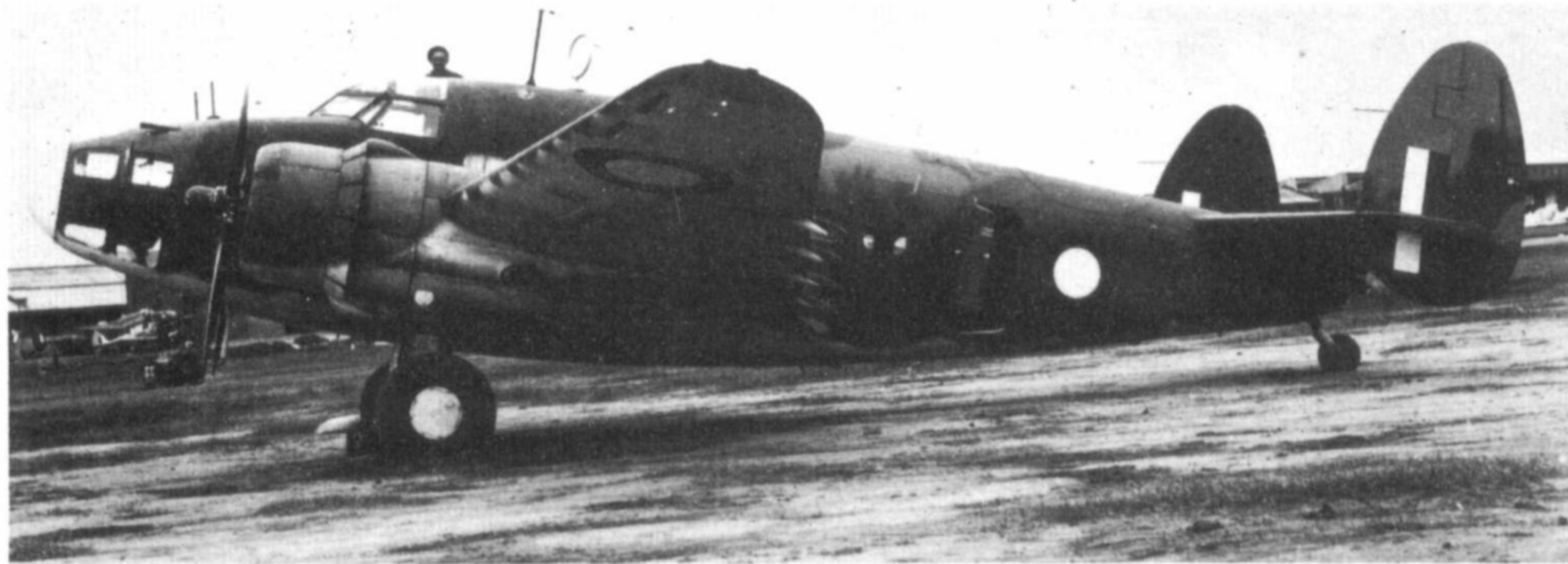
This Hudson Mk IVA (A16-143) was photographed at No. 1 Aircraft Depot, Laverton, Victoria, in October 1943, and shows signs of various radar antennas. Subsequently, this Mk IVA flew as a radar laboratory with No. 1 Aircraft Performance Unit following further radar equipment modifications at No. 2 Aircraft Depot, Richmond, NSW. No serials under wings. (Photo: Richard Hourigan via F. F. Smith)
