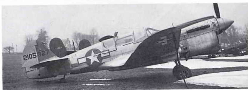
TP-40N in natural metal with OD anti-glare panel and fin, serial 2105927. (Roger F. Besecker).
