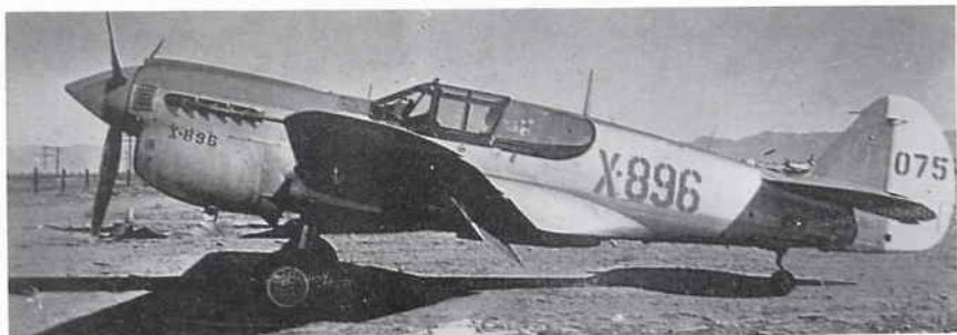
P-40L in natural metal with OD anti-glare panel, X-896 and fin, Serial 211075. (Peter M. Bowers).
