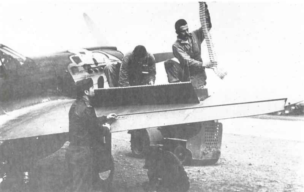
Above: P-40E of the 11th Fighter Squadron being re-armed, Unmak strip. Note filled-in exhaust aperture. (USAF).
