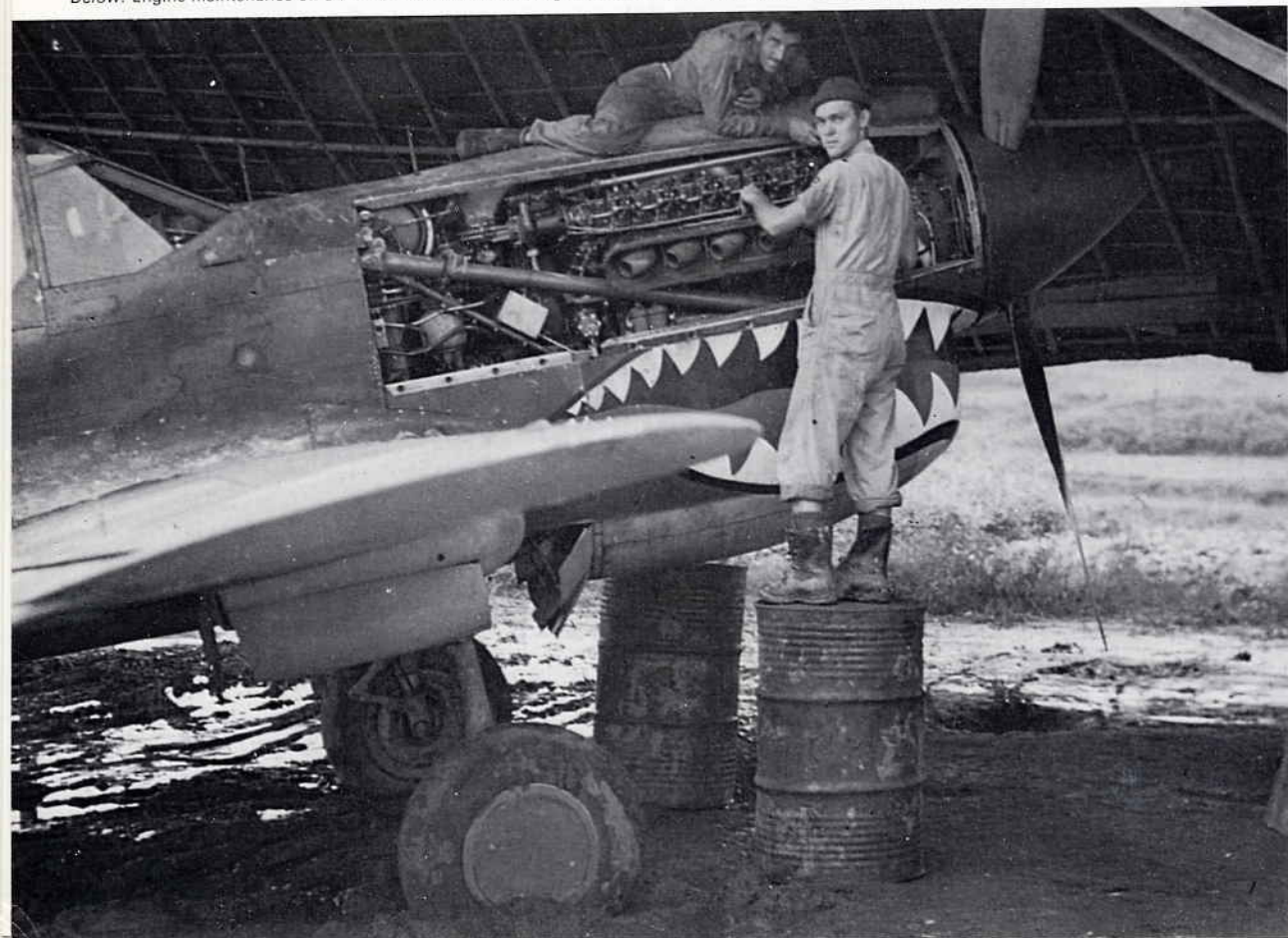
Below: Engine maintenance on a P-40K of the 51st FG being undertaken during the rainy season on an airfield in China. (USAF).
