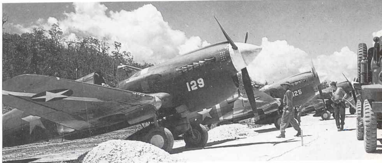
Above & below: P-40N 'Princess Pat II' being re-fueled at Munda airfield. Note non-standard drop tank, 18th FG 44th FS. (USAF).
