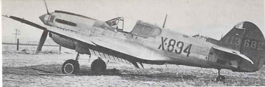
P-40R trainer (83rd P-40F re-engined). In natural metal with OD anti-glare panel, fin and rudder, red tip to spinner. (Peter M. Bowers).
