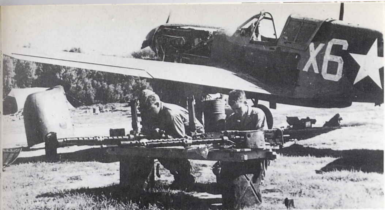
Armourers at work overhauling the '5's of a P-40F of the 79th Fighter Group, 87th Fighter Squadron on Castel Benito airfield. Note cowl under wing waiting for the application of the unit insignia. (USAF).
