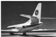
The first fan-engined Caravelle (c/n. 42) shown (above right) in original Series III form as F-WJAM, and (below) after re-registration as N420GE and re-engining with CJ805-23C's by General Electric.
