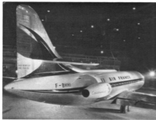
This nocturnal view of the prototype 02 shows the extreme simplicity of the original R.A.26 engine pods.
