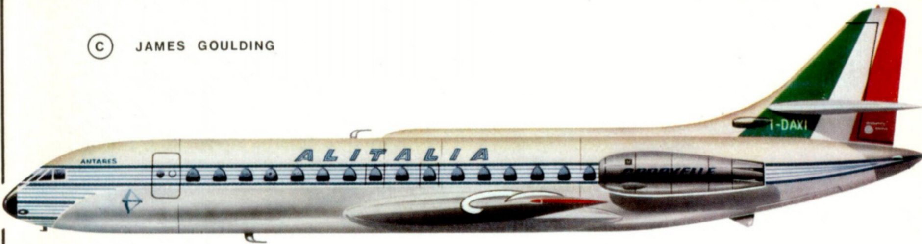
SUD-AVIATION CARAVELLE III, SE 210-40, I-DAXI "Antares" of Alitalia. This aircraft was later converted to Caravelle VI-N configuration.
