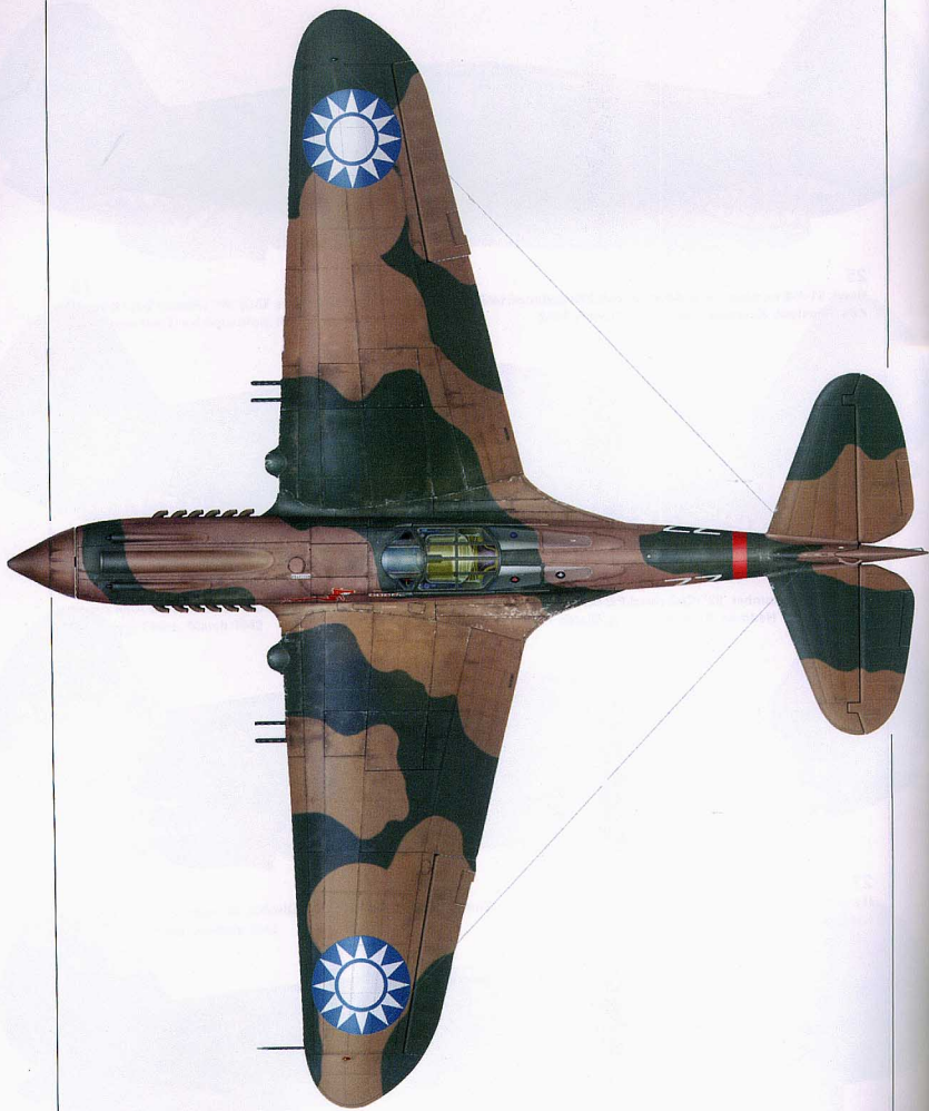
Upper plan view of Tomahawk '77', showing the camouflage pattern used on nearly all AVG Tomahawks. These shades were applied with the aid of rubber mats, insuring sharp demarcations and uniformity
